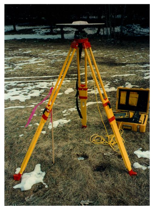
GPS base station used for differential correction. Notice that the antenna is located directly above a control point monument.
