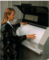
Vector digitizing with a tablet (left); raster digitizing with a drum scanner (right) (USGS). Compared to the drudgery of tablet digitizing, electronically scanning paper maps seems simple and efficient. Here's how CNSI describes it:
