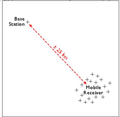
A GPS base station is fixed over a control point, while about 25 km away, a mobile GPS receiver is used to measure a series of positions.
