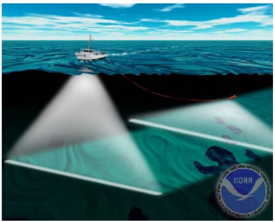
Multibeam and side scan sonar in use for bathymetric mapping. (NOAA, 2002). A <u>detailed report of the recent bathymetric survey of Crater Lake, Oregon, USA, is published by the USGS</u> here.
