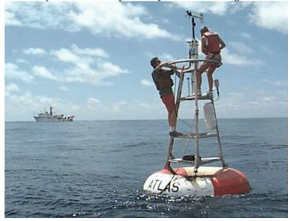
Researchers collect data from one of the 70 buoys in the Tropical Atmosphere Ocean (TAO) array. TAO buoys are equipped with sea surface temperature monitoring instruments. Hourly observations are stored in instrument memory and must be retrieved by operators. (Tropical Atmosphere Ocean Project, n. d.).
