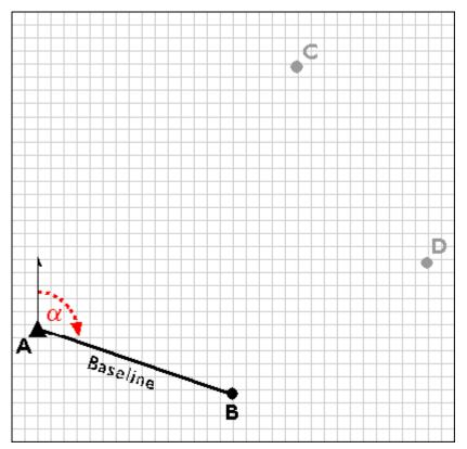
Establishing a second control point (B) in a triangulation network.
