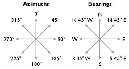
Azimuths and bearings.
