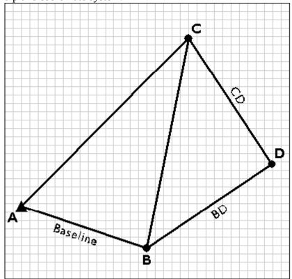
Fixing control point D by trilateration.
