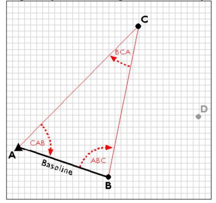
Establishing the position of point C by triangulation.
