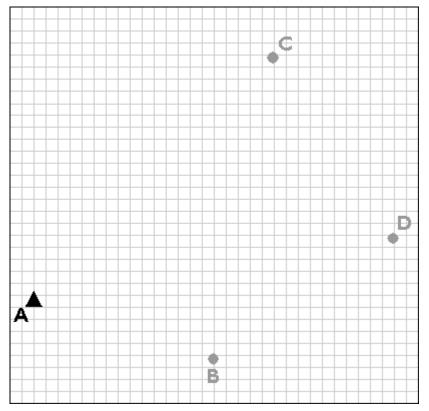
The purpose of a control survey is to establish new horizontal control points (B, C, and D) based upon an existing control point (A).
