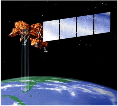
Artist's rendition of the Landsat 7 remote sensing satellite. The satellite does not really cast a four-sided beam of light upon the Earth's surface, of course. Instead, it merely records electromagnetic energy reflected or emitted by the Earth. (NASA, 2001).
