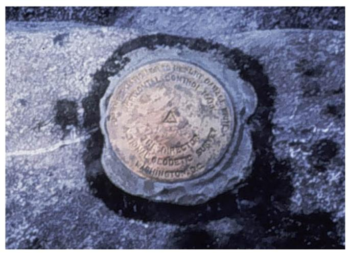
In the U.S., high-order horizontal control point locations are marked with permanent metal "monuments" like the one shown above. The physical manifestation of datum is a network of control point measurements (National Geodetic Survey, 2004).
