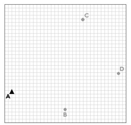
Trilateration is used to extend control networks by establishing new control points (B, C, and D) based upon existing control points (A).
