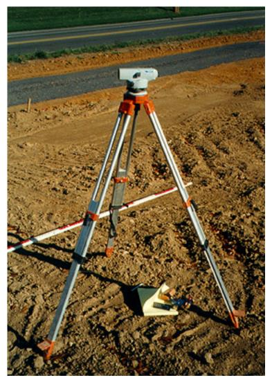
A level used for determining elevations.
