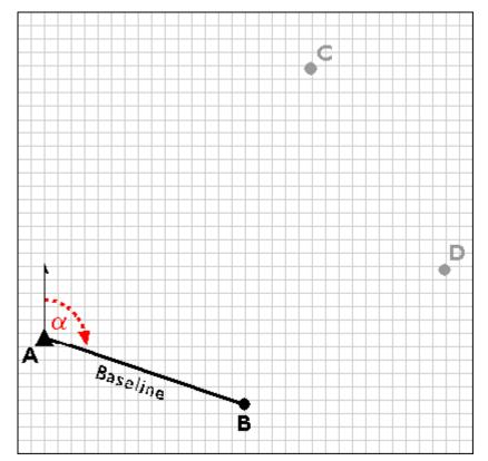
Establishing a second control point (B) in a trilateration network.
