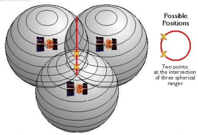
Set of possible positions of a GPS receiver relative to three GPS satellites. (Adapted from Hurn, 1993).
