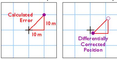
Error correction calculated at the base station is applied to the position calculated by the mobile receiver.
