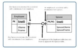
Figure 9.9. Example usage of a zero to one optional relationship symbol, by A. Watt.
