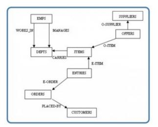
Figure 4.1. Network model diagram.
