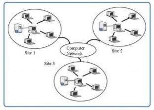
Figure 6.2. Example of a distributed database system.
