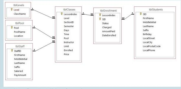
Figure 9.17. ERD for questions 1-5. (Diagram by A. Watt.)
