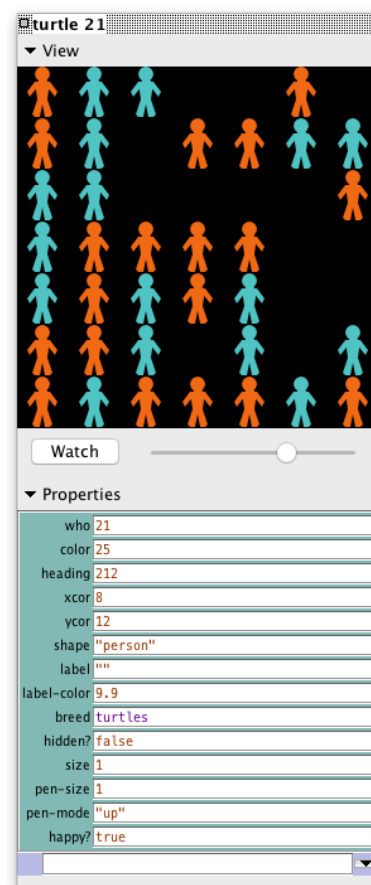
Figure 5. Window that pops up when you inspect a turtle. You can ask the turtle to execute instructions by typing them on the bottom line.
