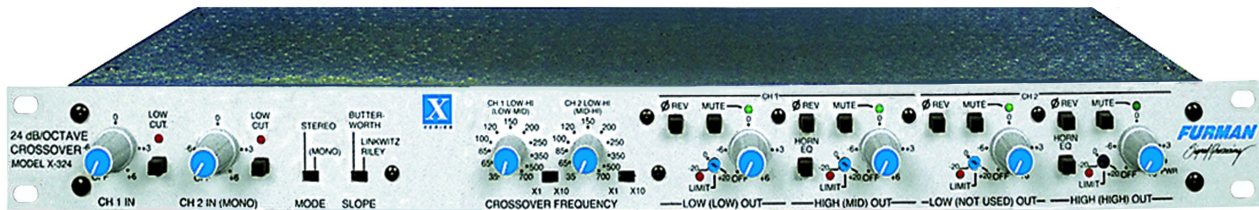
Figure 11.32 Commercial electronic crossover Reprinted courtesy of Furman Sound, Inc.
