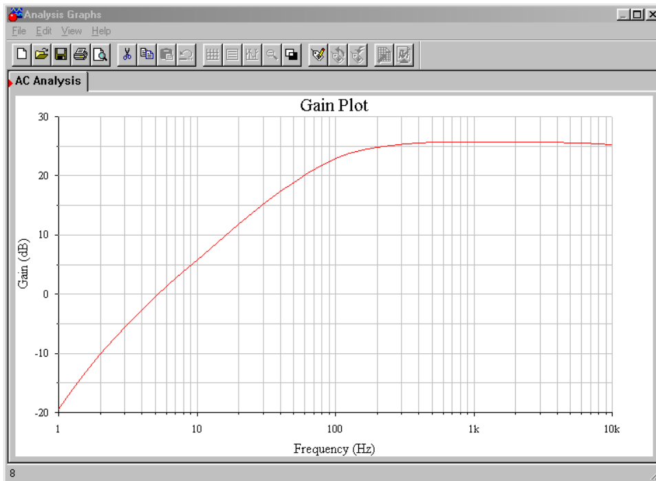
Figure 6.28b Gain plot for LM3900 amplifier
